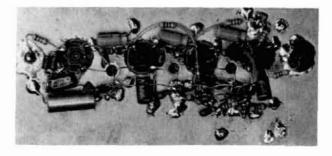
fig. 2. Single-sided solder tack construction technique is fast and mechanically/electrical sound. A few circuit improvements have been made so schematic differs slightly.
